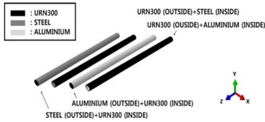
Fig. 2. Four types of hybrid pantographs for the parametric study
