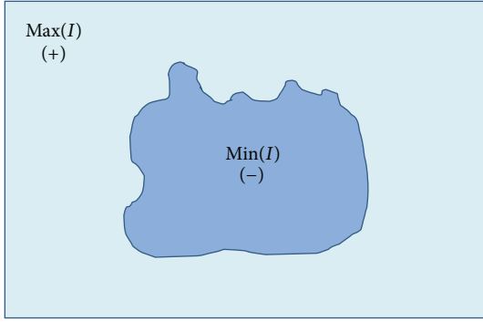
FIGURE 2: The signs of the SPF function inside and outside the object are opposite one another.
