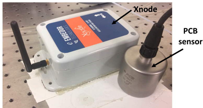
Figure 14. Ambient vibration test in an optical table.
