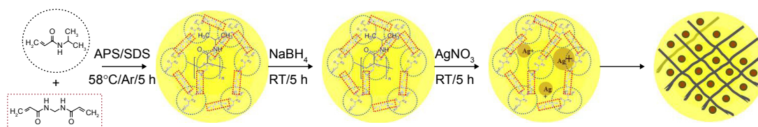
Figure 2 Schematic diagram of the synthesis of silver nanoparticle (AgNP)-encapsulated poly- N -isopropylacrylamide (pNIPAM)-based nanoparticle platforms. Abbreviations: APS, ammonium persulfate; RT, room temperature; SDS, sodium dodecyl sulfate.
