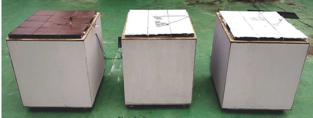
FIGURE 8: Scale-model experiment finish colors (Test 2).
