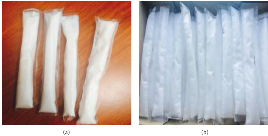
FIGURE 2: Packing-type PCM: (a) Bio 26°C CPCM, (b) RT 44°C PCM.
