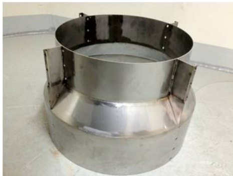
Fig.8. Mock-Up Model of the Multi-Diffuser
