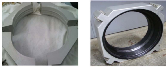
Assembly of Al-mould and Composite stacking
