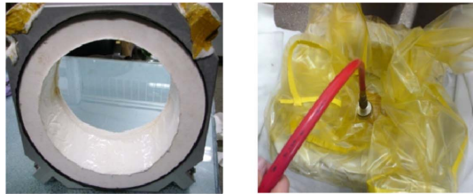
Assembly of inner mould and Degassing
