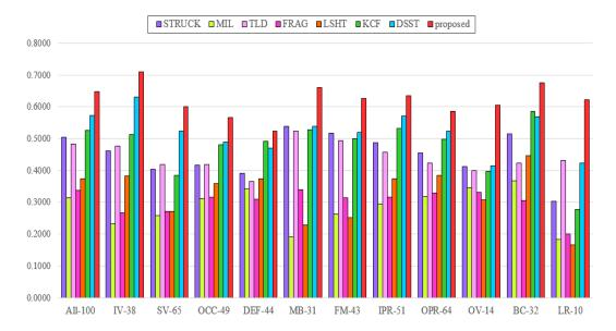
**Figure 7.** The average success rate of the proposed tracker and existing trackers with all attribute sequences in OTB-100. The number indicates the number of sequences including attributes; illumination variation (IV), scale variation (SV), occlusion (OCC), deformation (DEF), motion blur (MB), fast motion (FM), in-plane rotation (IPR), out-of-plane rotation (OPR), out-of-view (OV), background clutter (BC) and low-resolution (LR).
