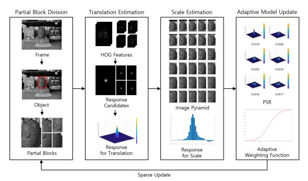
**Figure 2.** The block diagram of the proposed method. We separate the partial blocks from the object in the frame and perform the translation estimation and scale estimation. Finally, we perform the model update with the weighting function or skip the update. PSR, peak-to-sidelobe ratio.
