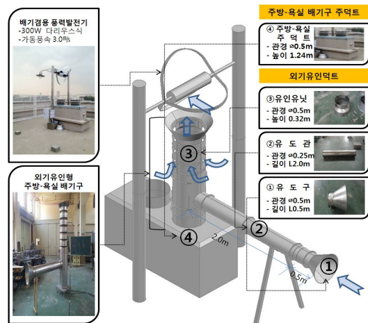
Fig. 1 Conceptual scheme of external induction-style kitchen and bathroom vents
