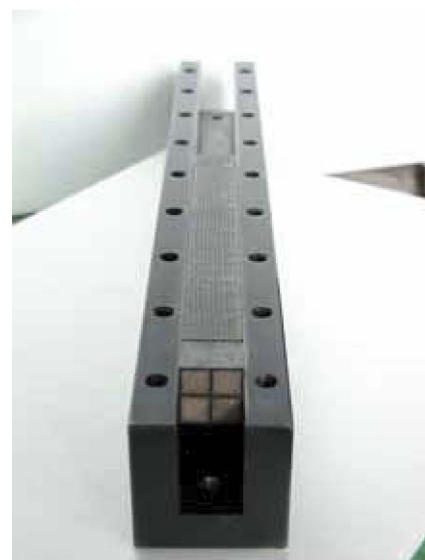
Fig. 11. Fabrication of the sandwich column with a mould.
