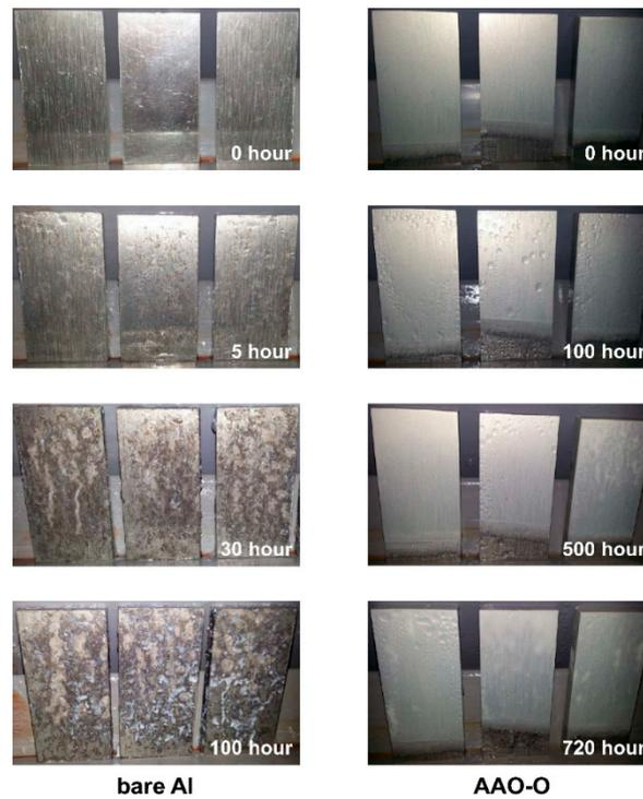
**Figure 6.** Results of salt spray test for bare aluminum and AAO-O (oil impregnation on anodic aluminum oxide) surfaces.
