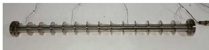
Figure 5. Photograph of the fabricated annular finned tube.
