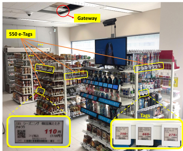
FIGURE 1. A picture of our 550-tag real convenience store deployment. A gateway is mounted on the ceiling, and there are 550 e-tags on the shelves displaying real product information.
