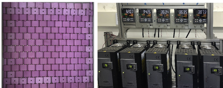
Fig. 15. Ceramic bend heater and PID system.
