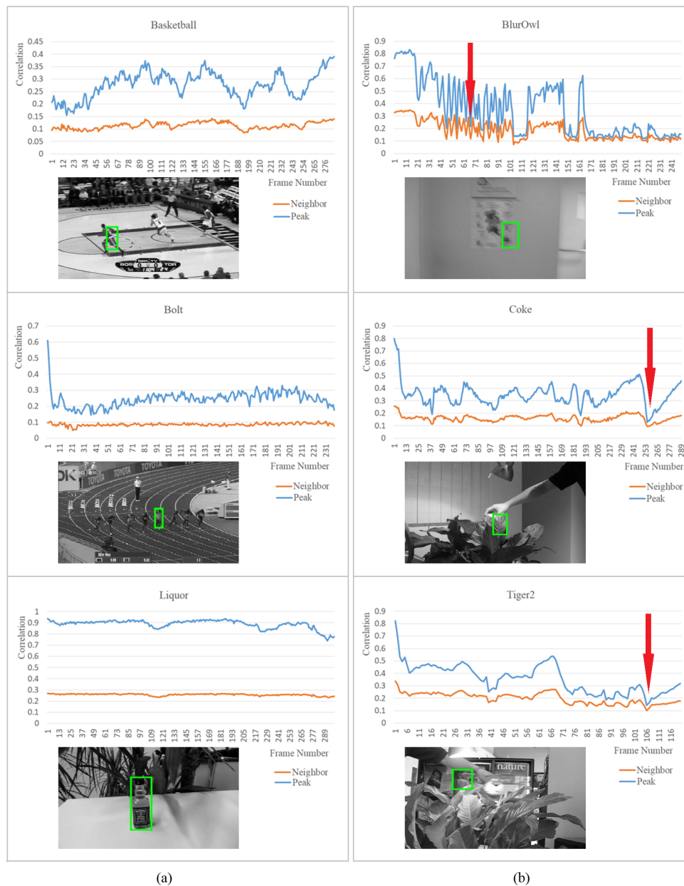
Figure 3. Comparison of peak values and average values of neighbor area around the peak. (a) Correlation developments with successfully tracked targets. (b) Correlation developments in sequences including tracking failures.
