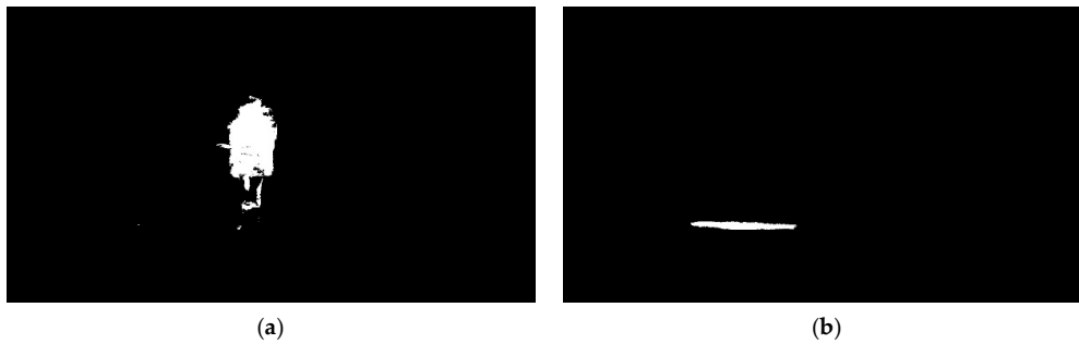
Figure 3. Example of shadow extraction in image sequence 1: (a) segmented object and (b) shadow region.
