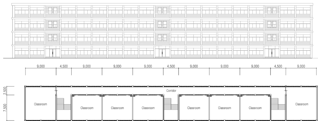
(a) Standardized school building and classroom arrangement in 1975 [9]
