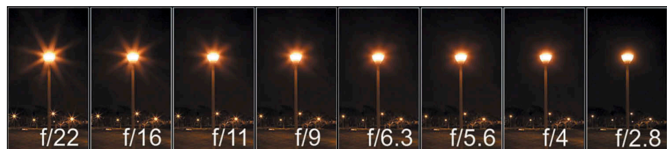
Figure 22. Label: Variation in light spread from illumination source owing to changes in aperture.
