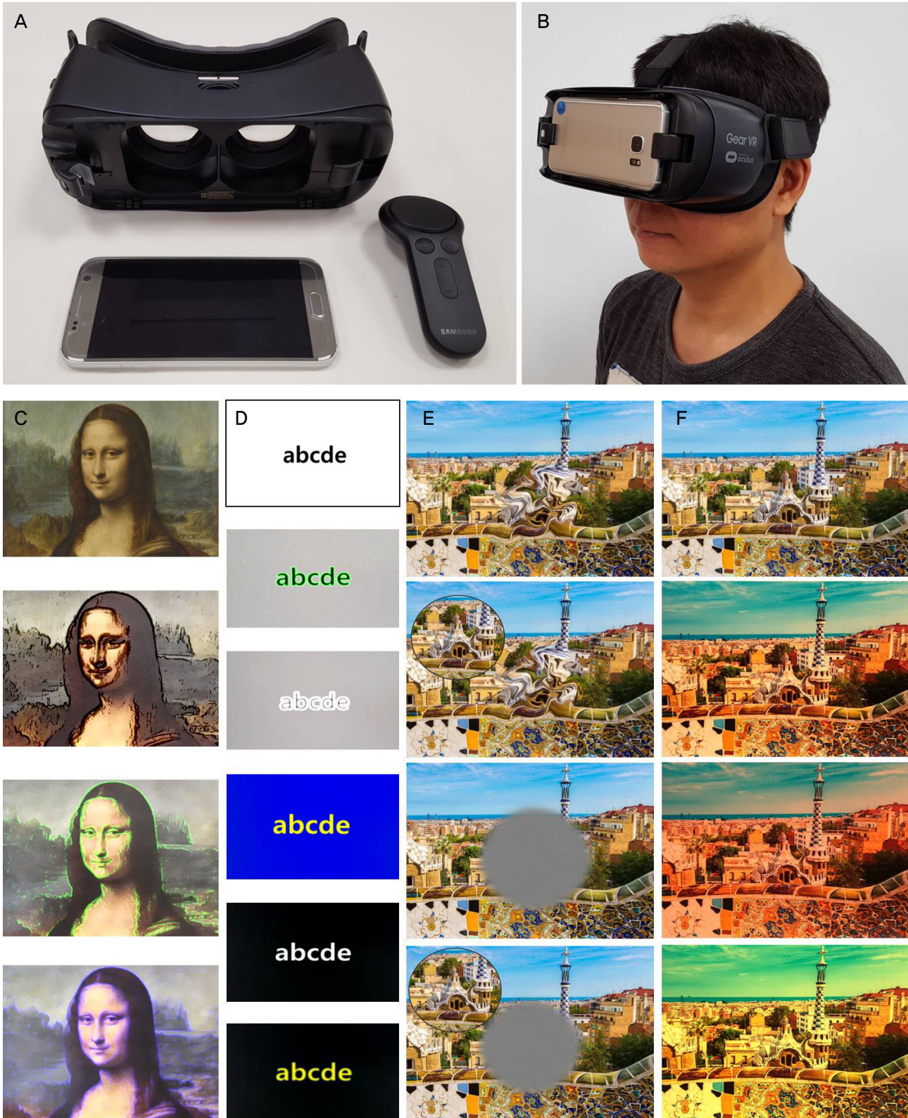
Figure 1. The low vision aid using virtual reality device (LVA-VR) that is capable of simultaneously performing multiple functions. (A) The LVA-VR is composed of the VR head-mounted display, a smartphone, smartphone application software, and a remote control. (B) Photograph of a patient wearing the LVA-VR. The operation remote is held in the patient's hand. The VLA-VR can perform edge enhancement (C), text enhancement (D), image remapping (E, moves central images to a more peripheral location), and color filtering (F). Each column begins with the original image and is followed by the enhanced images.
