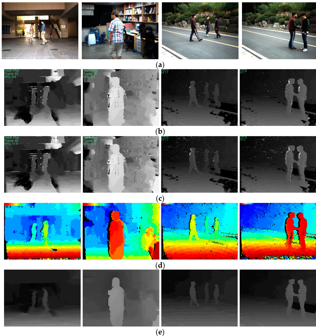
Figure 9. (a) Outdoor and indoor scene images; Disparity maps produced by (b) DCB grid [23]; (c) adaptive weight [21]; (d) MGM [24]; and (e) proposed method.
