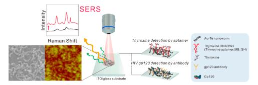
**Figure 1.** Schematic image of the fabricated biosensor platform. Note: SERS = surface-enhanced Raman spectroscopy, ITO = indium-tin-oxide.
