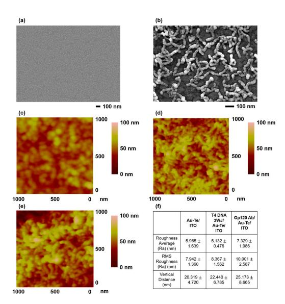
**Figure 2.** Field emission scanning electron microscopy (FE-SEM) image of (**a**) Bare indium-tin-oxide (ITO), (**b**) Au–Teon ITO. Atomic force microscopy (AFM) image of (**c**) Au–Te/ITO, (**d**) T4 DNA 3WJ/Au–Te/ITO, (**e**) GP120 antibody/Au–Te/ITO. (**f**) Surface roughness analysis of the Au–Te/ITO, T4 DNA 3WJ/Au–Te/ITO, and GP120 Ab/Au–Te/ITO (The surface roughness analysis was carried out at 10 different positions on the AFM images, respectively).
