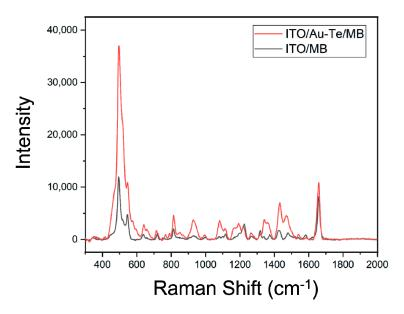
Figure 3. Raman spectrum of methylene blue on ITO, ITO/Au-Te.
