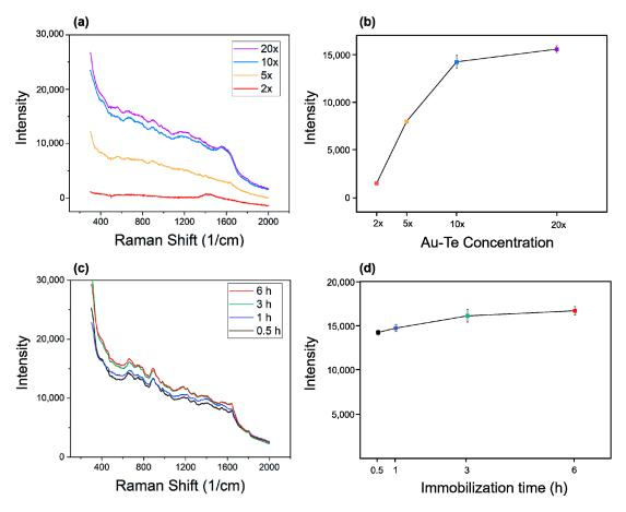
**Figure 4.** Optimum conditions for Au–Te immobilization on ITO. (**a**) Raman spectra of various Au–Te concentrations on an ITO substrate, (**b**) the SERS effect of Au–Te concentrations, (**c**) Raman spectra with different immobilization time conditions of Au–Te on ITO, (**d**) the SERS effect of Au–Te immobilization time.
