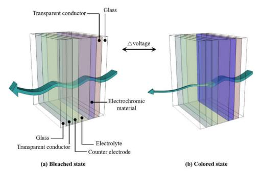
Figure 1. A schematic of a typical electrochromic window.
