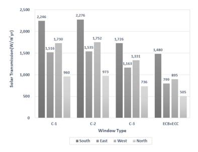
Figure 2. Annual solar transmission rate by orientation according to window type.
