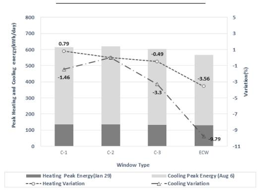
**Figure 12.** Peak Heating and Cooling energy consumption. (Variation: A percentage change compared to base model(C-2)).
