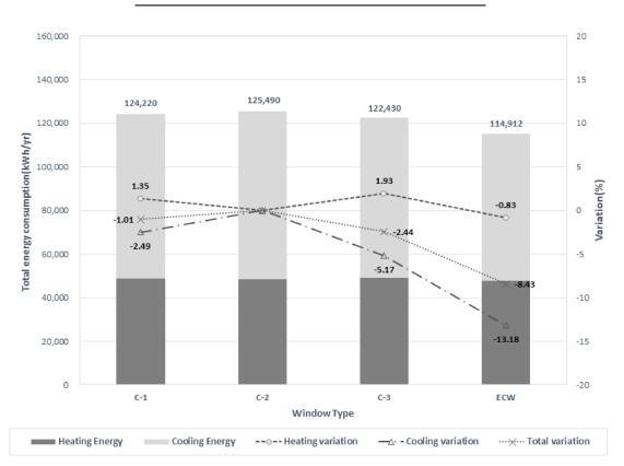
**Figure 11.** Annual heating and cooling energy consumption. (Variation: A percentage change compared to base model(C-2)).
