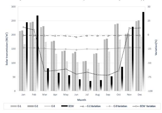
**Figure 3.** Solar transmission performance by direction (Monthly)—South. (Variation: A percentage change compared to base model(C-2)).
