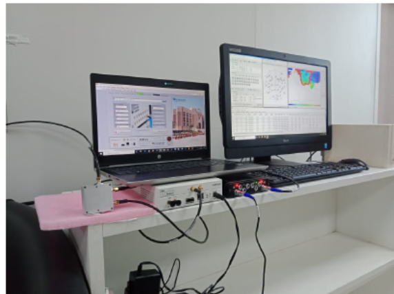
Figure 7. Experimental setup used for collecting GPS signals. The devices used in this experiment are Septentrio PolaRx5S GNSS receiver, USRP N210, splitter to split the signal between Spentrio receiver and USRP N210.
