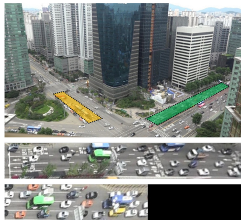
Figure 5. The original video snapshot (top), the green approach to train the former CNN model (middle), and the new yellow approach to test the transferability of the trained model (bottom). The new approach is zero-padded.
