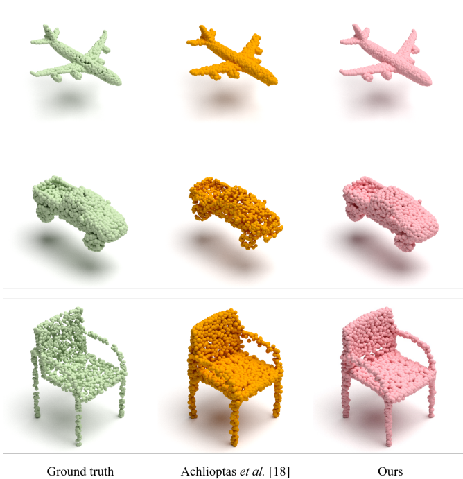
Fig. 4. Examples of reconstructed point clouds by autoencoder. From top to bottom: airplane, car, and chair. From left to right: ground truth, PointNet-based autoencoder [18], and our LDGCNN-based autoencoder.
