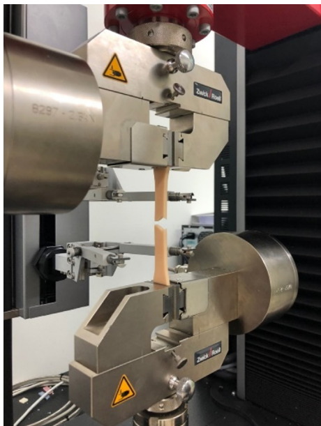
Fig. 7. EP400 specimens during (left) and after (right) standard tensile test.
