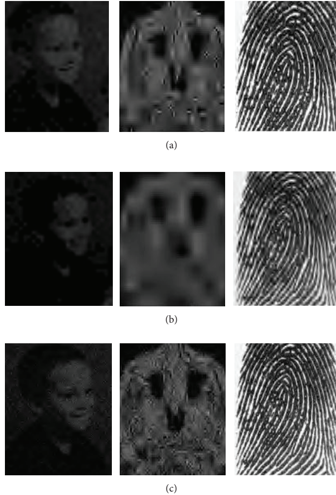
FIGURE 5: Local enlarged denoising images. (a) The hard threshold denoising algorithm. (b) The soft threshold denoising algorithm. (c) The improved wavelet threshold algorithm.
