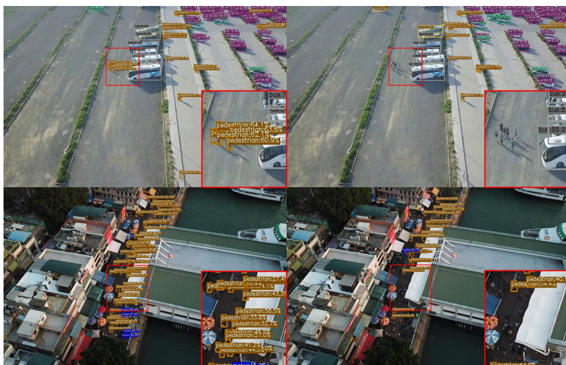
Figure 10. Subjective comparison of small object detection performance: (left) our network with Input_size 1280, and (right) YOLOX-s with Input_size 640.
