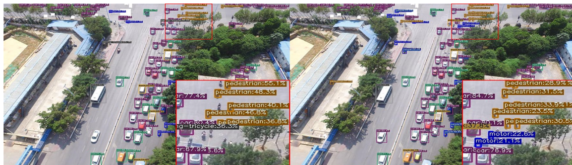
Figure 8. Subjective comparison of small object detection performance: (left) original YOLOX-s model with Input_size 640, and (right) our network with Input_size 1280.
