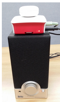
FIGURE 1. A speaker prototype with a beacon and a Raspberry Pi.
