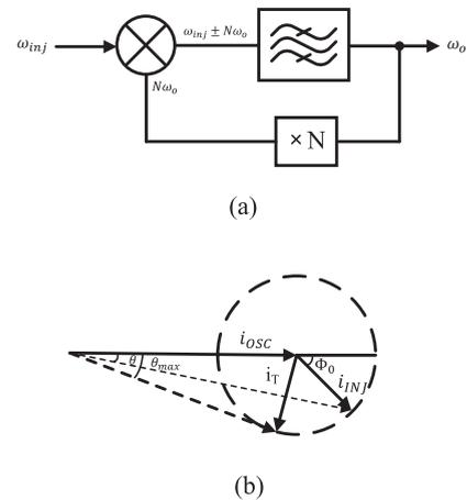
FIGURE 2. (a) Block diagram of harmonic ILFD. (b) phase diagram of injection-locked oscillator/divider.
