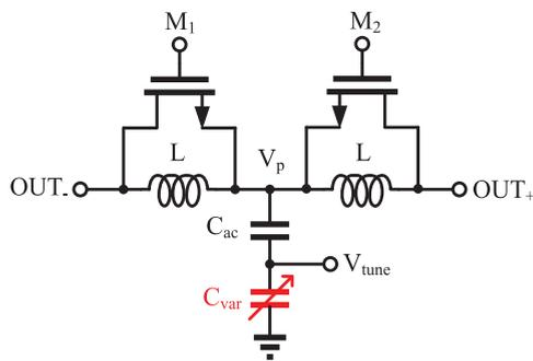
FIGURE 4. Phase tuner with T-network.
