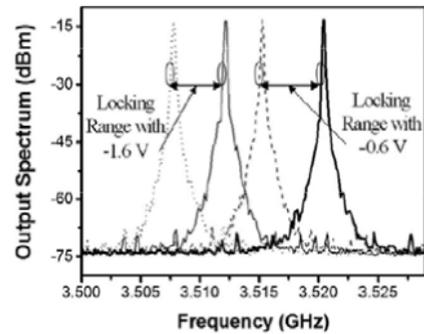
FIGURE 17. Measured output spectrum ( $P_{inj} = -18\text{dBm}$ ) with non-optimal ( $V_{tune} = -1.6\text{V}$ ) and optimal ( $V_{tune} = -0.6\text{V}$ ) phase tuning voltage of the 11.1-GHz divide-by-3 ILFD.
