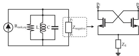
FIGURE 3. Equivalent circuit of the resonator with negative resistance due to cross-coupled transistors.
