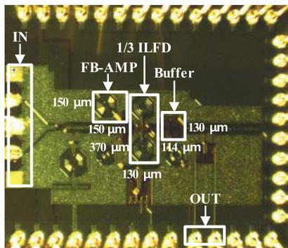
FIGURE 11. 11.7GHz divide-by-3 ILFD test chip photograph.
