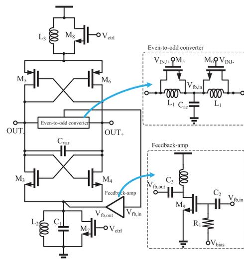
FIGURE 8. Schematic of the 11.7-GHz divide-by-3 ILFD.
