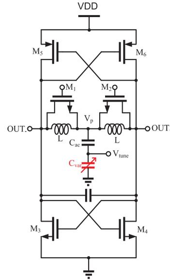
FIGURE 7. Schematic of the 11.1-GHz divide-by-3 ILFD.
