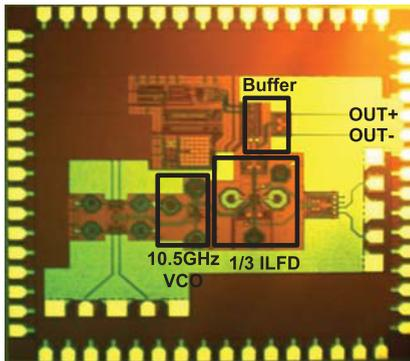
FIGURE 10. 11.1GHz divide-by-3 ILFD test chip photograph.
