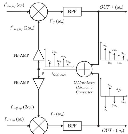
FIGURE 5. Block diagram of the divide-by-3 ILFD utilizing self-injection with odd-to-even harmonic converter.
