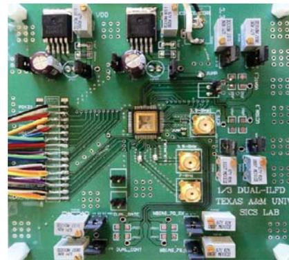
FIGURE 14. 11.7GHz divide-by-3 ILFD test chip packaged and mounted on FR-4 board.
