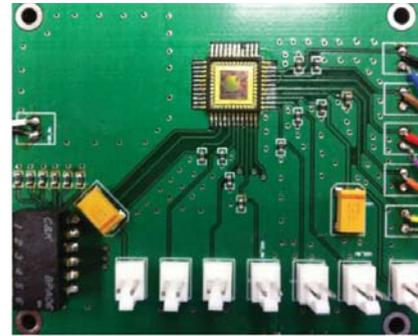
FIGURE 12. 7.8GHz divide-by-2 ILFD test chip packaged and mounted on FR-4 board.
