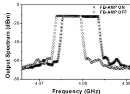
FIGURE 19. Measured locking-range ( $P_{inj} = -12\text{dBm}$ ) with feedback path on and off of the 11.7-GHz divide-by-3 ILFD.
