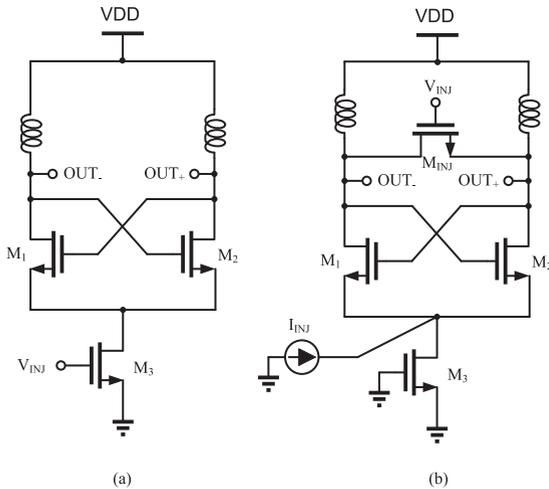
FIGURE 1. Conventional ILFD: (a) tail injection method. (b) direct injection method.
