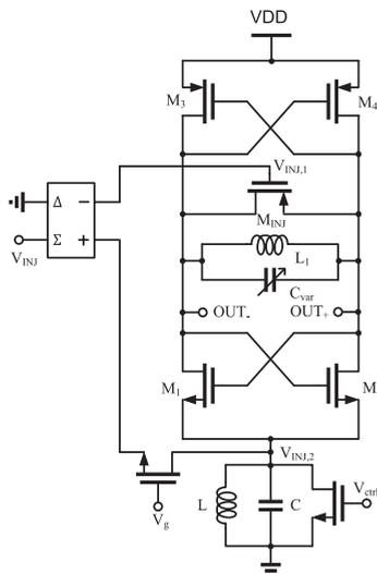
FIGURE 6. Schematic of the 7.8-GHz divide-by-2 ILFD.
