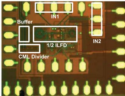
FIGURE 9. 7.8GHz divide-by-2 ILFD test chip photograph.
