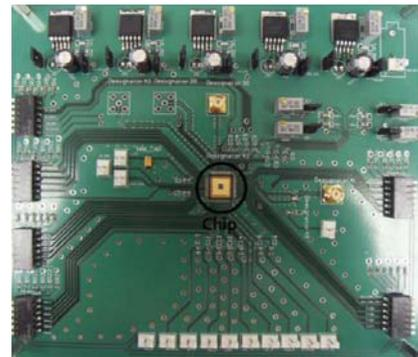
FIGURE 13. 11.1GHz divide-by-3 ILFD test chip packaged and mounted on FR-4 board.
