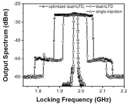
FIGURE 15. Measured locking-range ( $P_{inj} = 10\text{dBm}$ ) of the 7.8-GHz divide-by-2 ILFD.
