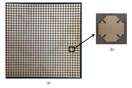
Figure 5. Pictures of (a) fabricated metamaterial absorber prototype and (b) enlarged view of a unit cell.
