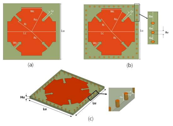
**Figure 1.** Unit cells of the proposed absorber (**a**) without via array, (**b**) with via array, and (**c**) 3D view of (**b**) (unit: mm)  $L_u = 8$ ,  $L_c = 6.8$ ,  $R_o = 3.3$ ,  $R_i = 2.4$ ,  $R_c = 2.05$ ,  $W_r = 0.9$ ,  $W_c = 2.9$ ,  $G_c = 0.3$ ,  $R_v = 0.2$ ,  $G_o = 0.75$ ,  $G_v = 0.5$ , and  $H_u = 0.35$ .
