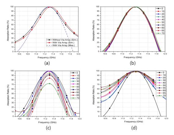
**Figure 7.** (a) Simulated and measured absorptivity of the metamaterial absorber with and without the via array under normal incidence. (b) Measured absorptivity of the fabricated absorber sample for different polarization angles ( $\varphi$ ) under normal incidence. Measured absorptivity of the fabricated absorber sample for different incident angles ( $\theta$ ) under (c) TE mode and (d) TM mode.
