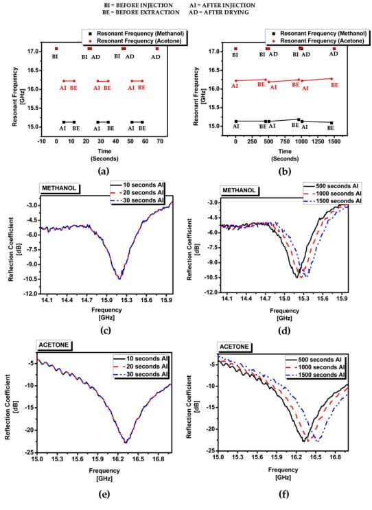
**Figure 8.** Repeatability test of the proposed SIW chemical sensor for methanol and acetone: (a) frequency variation of test #1 (fast injection and extraction process); (b) frequency variation of test #2 (slow injection and extraction process); (c) measured reflection coefficients of test #1 with methanol; (d) measured reflection coefficients of test #2 with methanol; (e) measured reflection coefficients of test #1 with acetone.
