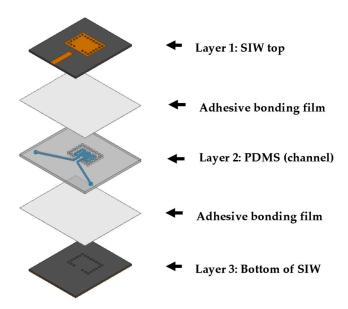
Figure 3. Layers of the proposed SIW chemical sensor.
