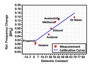
Figure 9. Sensitivity of the proposed SIW chemical sensor.
