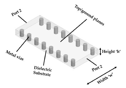
Figure 1. Illustration of SIW structure.
