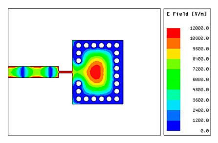
Figure 2. Electric field distribution of a SIW cavity resonator.
