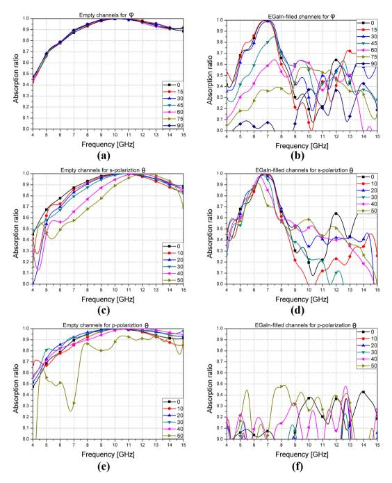
**Figure 6.** Measurement results at different polarization ( $\varphi$ ) and incident ( $\theta$ ) angles for s-and p-polarization: (**a**) Empty channels and (**b**) EGaIn-filled channels for  $\varphi$ . (**c**) Empty channels and (**d**) EGaIn-filled channels for s-polarization  $\theta$ . (**e**) Empty channels and (**f**) EGaIn-filled channels for p-polarization  $\theta$ .
