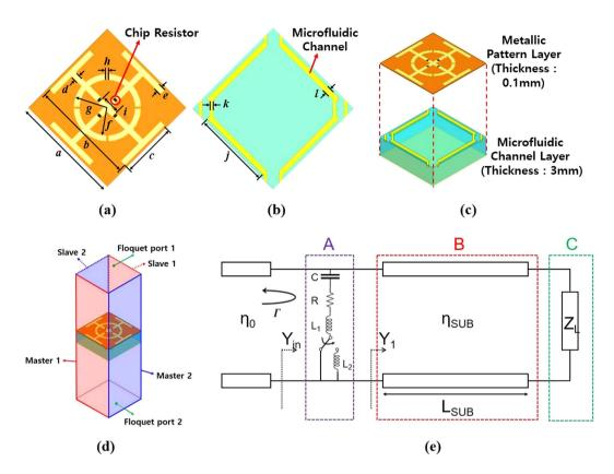
Figure 1. The unit cell of the proposed absorber: a = 10 mm, b = 9.5 mm, c = 5 mm, d = 0.5 mm, e = 0.5 mm, f = 2.5 mm, h = 0.2 mm, h = 1.74 mm, h = 1.74 mm, h = 0.3 mm, h = 0.5 mm. (a) JC resonator with slotted circular ring and chip resistors. (b) Microfluidic channels. (c) Three-dimensional view of the unit cell. (d) Boundary conditions and excitations for a periodic structure. (e) Transmission line model of the proposed absorber.
