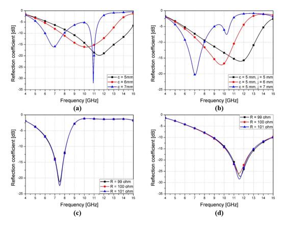
**Figure 3.** Simulation results for (a) different lengths of c without the microfluidic channels, (b) different lengths of j without the microfluidic channel connection, (c) EGaIn-filled channels and (d) empty channels with  $\pm 1\%$  variation of resistance.
