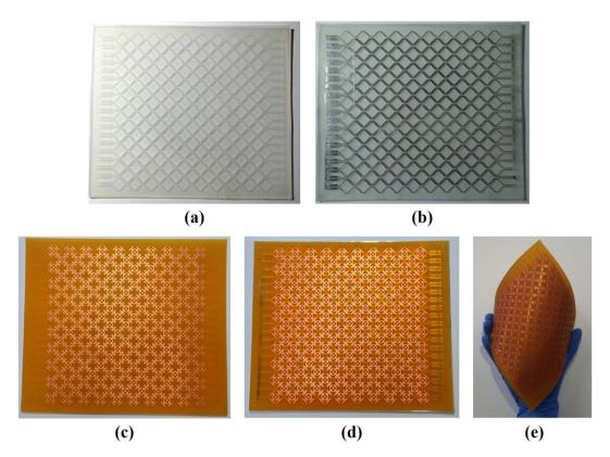
**Figure 2.** Fabricated microfluidic channel: (a) Empty state. (b) EGaIn filled state. Fabricated prototype of the proposed absorber with (c) empty channels, (d) EGaIn-filled channels and (e) folded sample.
