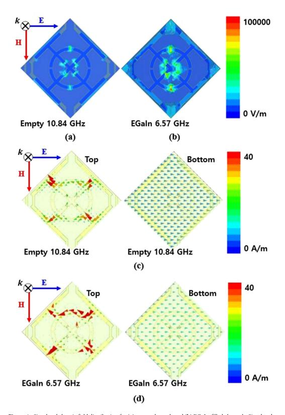
**Figure 4.** Simulated electric field distribution for (a) empty channels and (b) EGaIn-filled channels. Simulated vector current distribution for (c) empty channels, and (d) EGaIn-filled channels.
