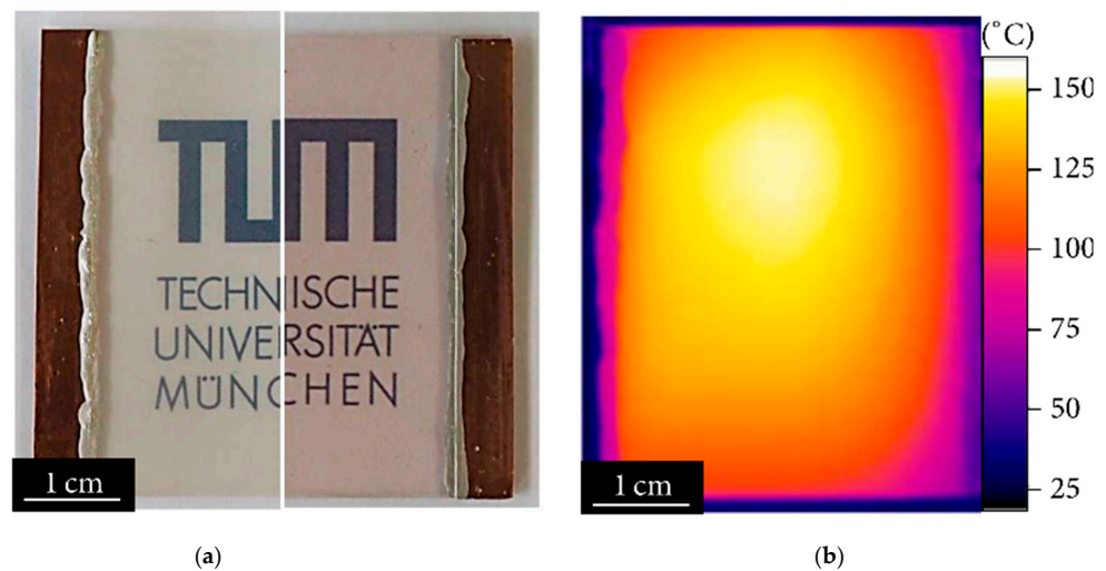
Figure 7. Optical microscope image of an AgNW-based transparent heater. (a) shows the highly transparent AgNW layer on the glass substrate; (b) the uniform and efficient heating performance. Reproduced from Ref. [51] under the Creative Commons Attribution 4.0 International (CC BY 4.0) License.
