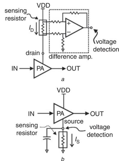
Fig. 3 Voltage detection by sensing resistor to monitor resonance variations
