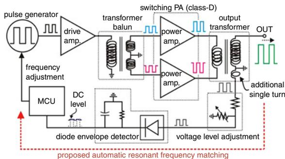
Fig. 1 Structure of proposed automatic resonant frequency matching circuitry by searching minimum DC-level
