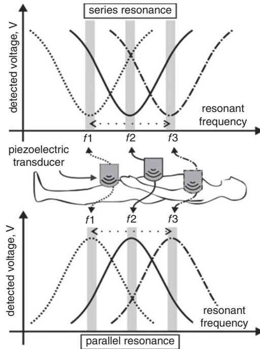
Fig. 2 Variations in resonant frequency with respect to different contact points on human body
