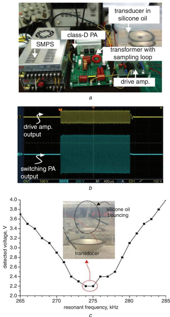
**Fig. 4** Implementation and measured results of proposed structure with ultrasonic transducer
