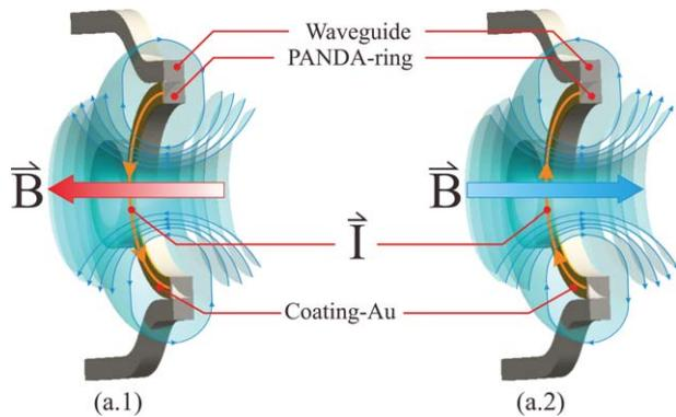
**Figure 5** Shows a schematic diagram of magnetic field (current), where the Au is the coated material. [Color figure can be viewed in the online issue, which is available at [wileyonlinelibrary.com](http://wileyonlinelibrary.com)]
