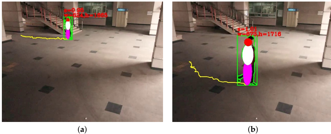
Figure 11. Size estimation results of the same object that is (a) far from the camera; (b) close to the camera.
