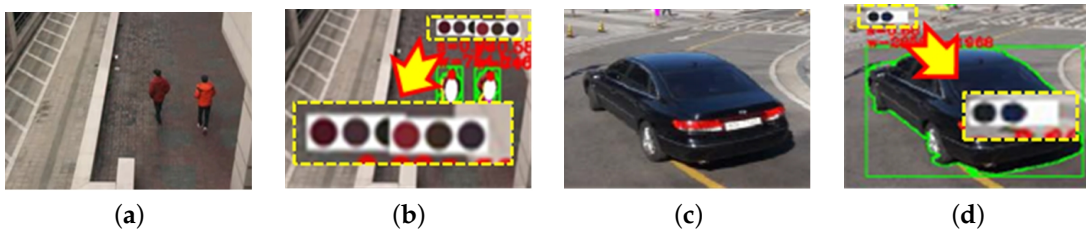
Figure 10. Selection of the representative colors from the candidate colors computed by the K-means clustering algorithm: (a) input image with two people; (b) the result of color selection; (c) an input image with a vehicle; (d) the result of color selection.
