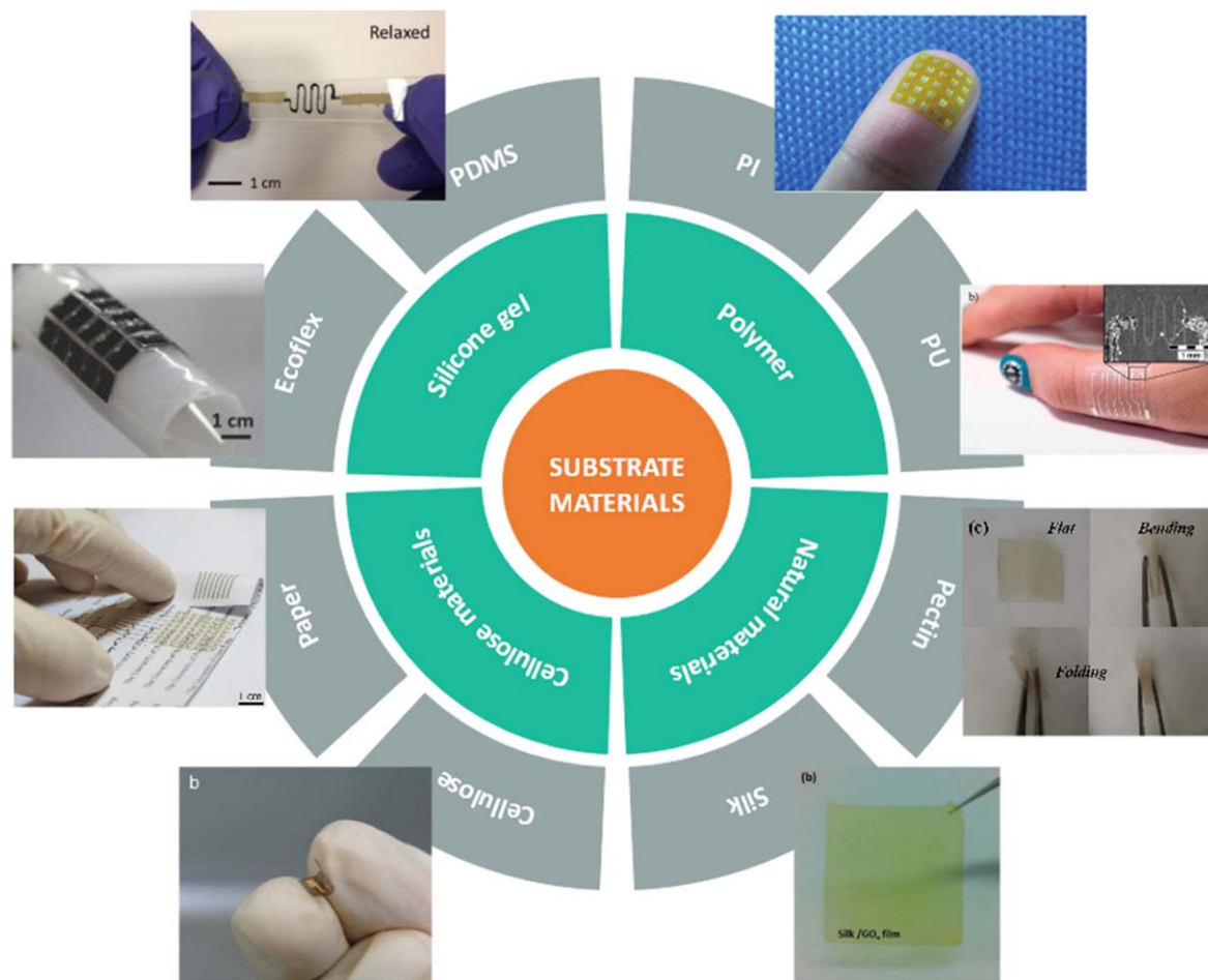
Figure 1. Schematic illustration of the substrate materials for parts of flexible sensors. Clockwise from top right: polyimide (PI), polyurethane, pectin, silk, cellulose, paper, ecoflex, and polydimethylsiloxane. Reproduced from [34] under the Creative Commons Attribution 4.0 International (CC BY 4.0) Licence.
