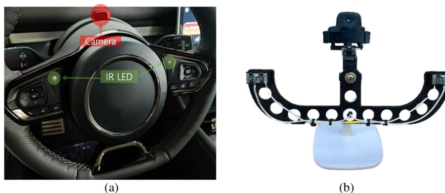
Figure 3. DMS camera in CANLAB: (a) DMS camera mounted on a vehicle and (b) prototype of the DMS camera.
