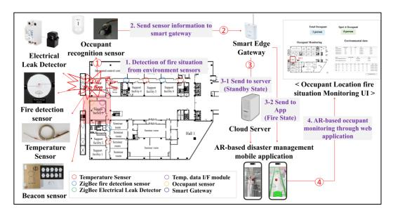
Figure 13. SFSMS mobile/web application data flow.
