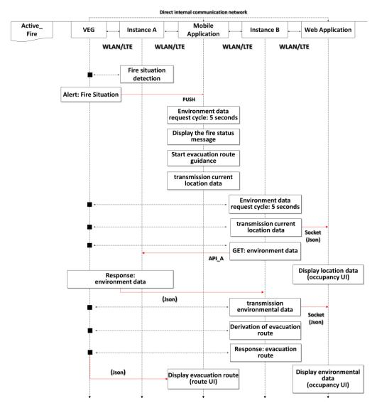
Figure 11. System status: active\_fire data flow.
