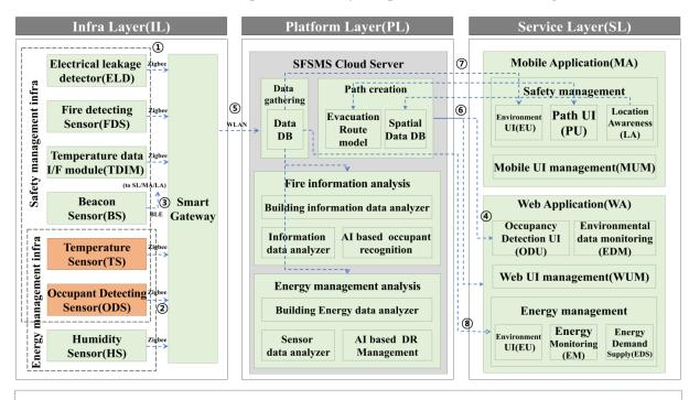
Zigbee network-based fire environment data transmission ② Occupant's number detection ③ Occupant's location detection ④ Deep learning-based video occupant recognition ⑤ WLAN network-based fire environment data transmission to server ⑥ Occupancy detecting simulation through Web application ⑦ AR based fire management simulation
