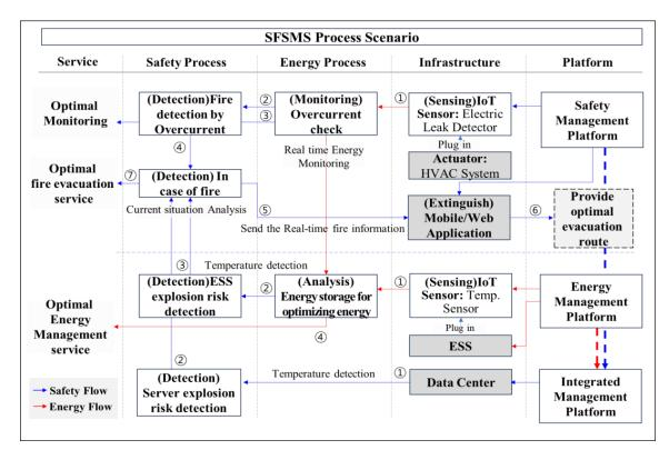
Figure 17. Safety and energy management control process scenario in SFSMS.
