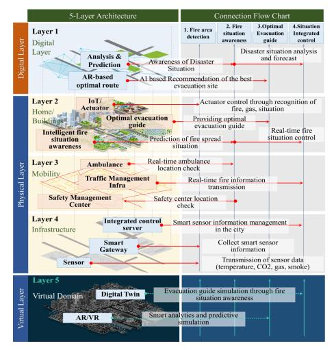
Figure 2. City-based 5-layer architecture.
