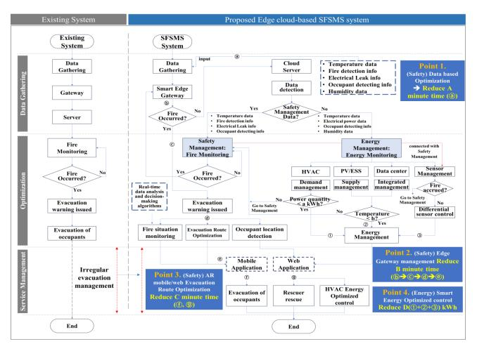
Figure 18. SFSMS algorithm compared to the existing system.
