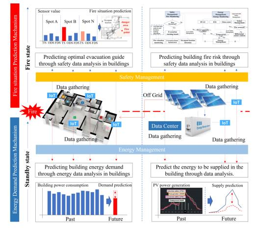
Energy management mainly comprises managing the HVAC, PV, and ESS and is operated in connection with the safety system when a fire occurs.
