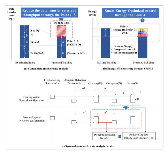
Figure 22. Four points for safety and energy management simulation results.
