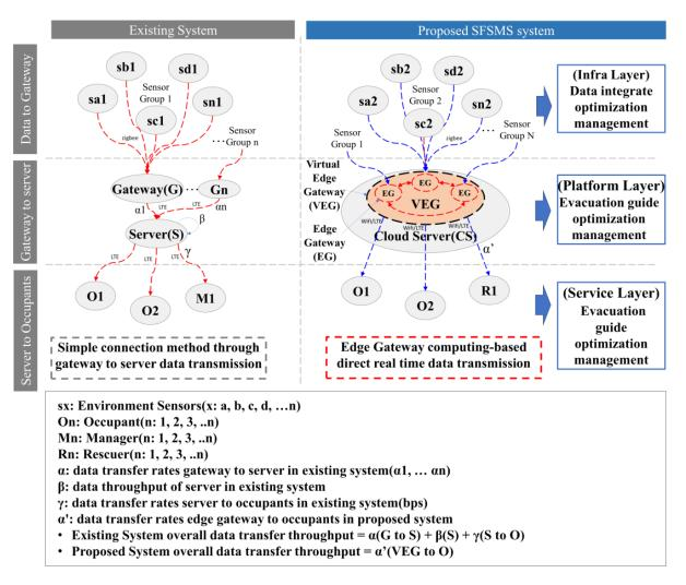
Figure 20. Point 2 for safety management of SFSMS compared to the existing system.
