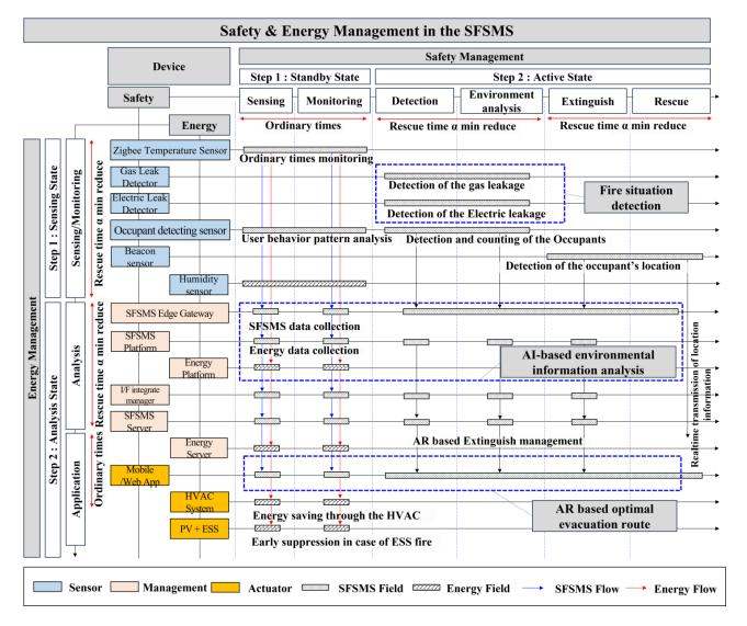
Figure 16. SFSMS process, including safety and energy management.
