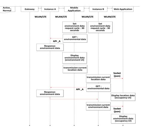
Figure 10. System status: active\_normal data flow.
