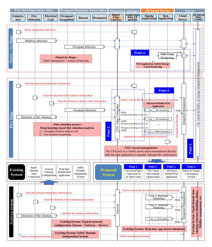
Figure 21. SFSMS data flow diagram compared to the existing system compared to the existing system.
