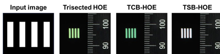
Figure 11. Experimental results of the three different types of SMDG HOE-based WG displays. Four white lines were adopted as the input image to quantitatively analyze the three colors detected by the CCD camera. The overlap of the physical object (the ruler) with virtual content (the white lines) showed that AR was implemented.
