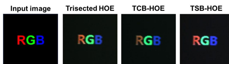
Figure 10. Captured experimental result image through the CCD camera after delivery via the three different types of SMDG HOEs-based WG displays. The input image (labeled RGB) served as the input for the beam projector.
