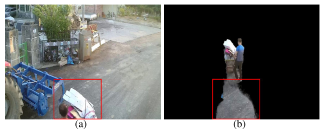
FIGURE 11. Illustration of matting inaccuracies when the initial background frame contains dynamic entities.
