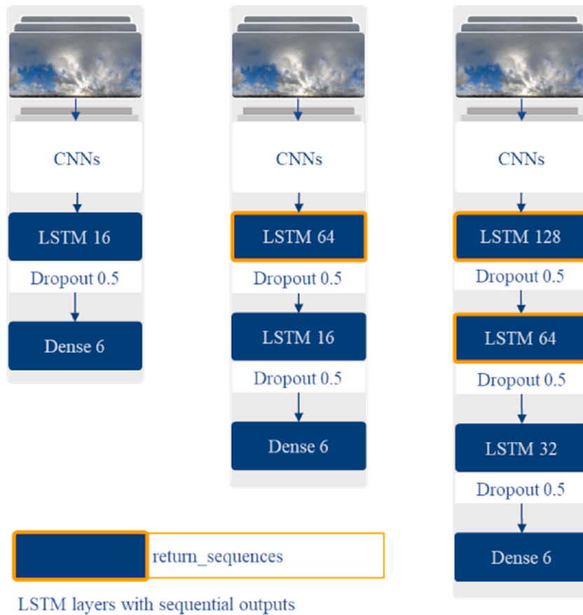
Fig. 6. Structures of LSTM stacks used in experiments.
