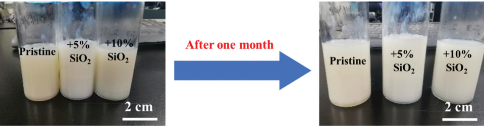
Figure 2. Optical photos of as-prepared water-based paints after keeping them standing for one month.
