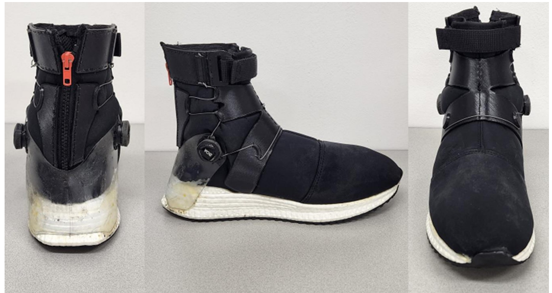
Fig 1. The prototype high-collar shoe was designed for this study. A wire connects two ratcheting reels to uniformly spread the pressure around the ankle. This design allows precise control over CAP by adjusting the ratcheting reels and top strap.
