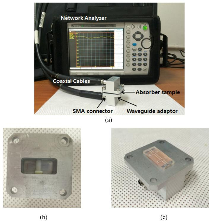
Fig. 8. (a) Waveguide measurement setup; (b) open-ended rectangular waveguide; (c) sample in the top of the waveguide adaptor.
