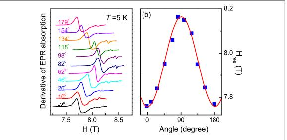
**Figure 5.** (a) Angular dependence of the EPR spectra (derivative of the absorption spectra versus field, vertically shifted for clarity) measured at  $\nu = 240$  GHz and at T = 5 K. (b) Angular dependence of the resonance fields. The solid line is a fit to the conventional expression  $H_{\text{res}} = \sqrt{H_{\perp} \sin^2 \theta + H_{\parallel} \cos^2 \theta}$ .
