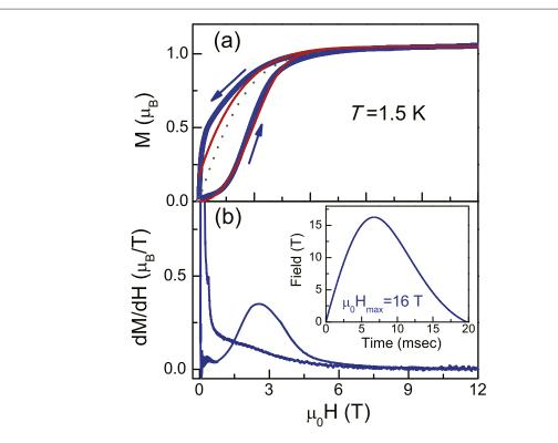
**Figure 3.** (a) Hysteresis loop (open circles) measured at T = 1.5 K using a fast sweeping pulsed field with a maximum field of  $\mu_0 H_{max} = 16$  T. The dotted line is the equilibrium magnetization measured by VSM. The red line is the simulated magnetization curve. (b) Derivative dM/dH of the magnetization curve. The sharp peak at zero field in dM/dH corresponds to magnetization jump. The inset plots the time dependence of a pulsed magnetic field.
