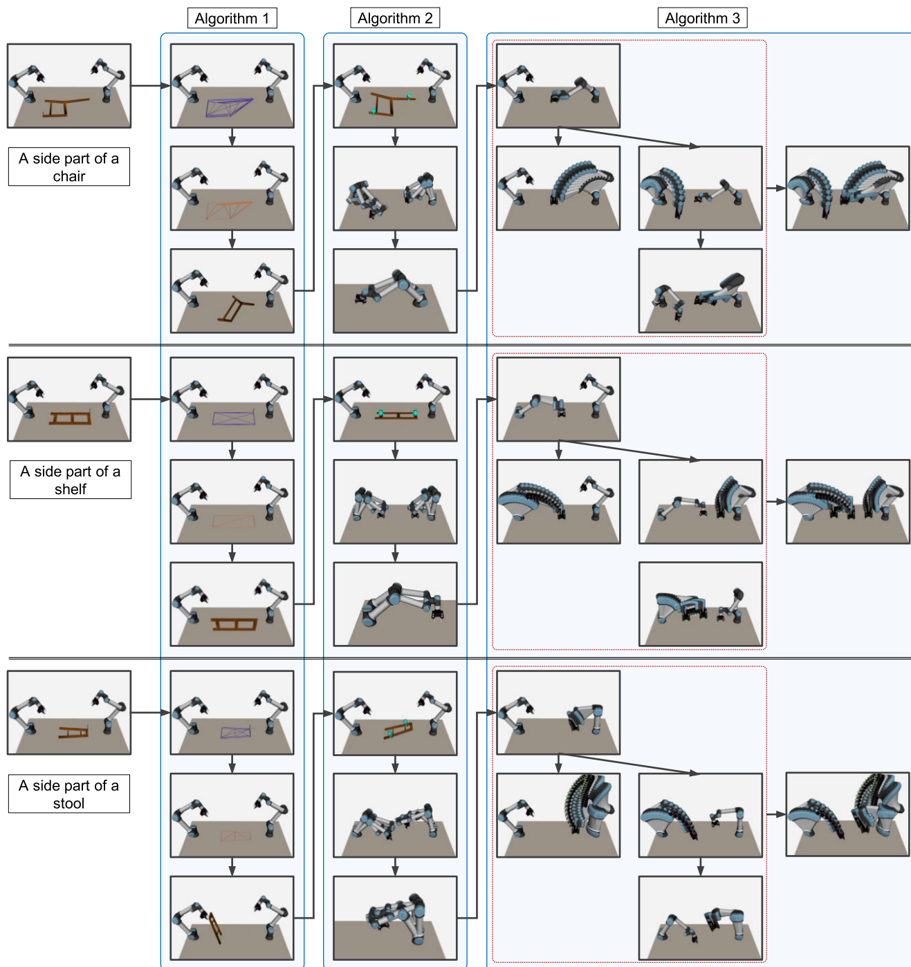
FIGURE 7. Examples of applying algorithms to objects in the simulation: a side part of a chair, of a shelf, and of a stool. The rows present the process of the algorithms for each object, and the columns show snapshots of applying each algorithm to the object.
