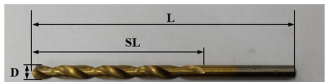
FIGURE 3. Detailed dimension of drilling tool (HSS, 135° drill point angle, 61mm (L) × 33mm (SL)×3mm (D); 75mm (L) × 43mm (SL) × 4mm (D)).
