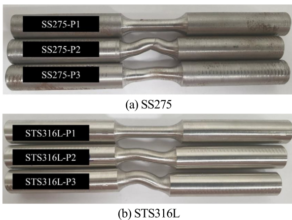
Fig. 8. Failure shapes of cyclic coupons at test ends.
